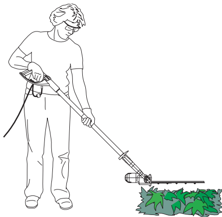
Figure 16 - Trimming Low Foliage or Ground Cover
